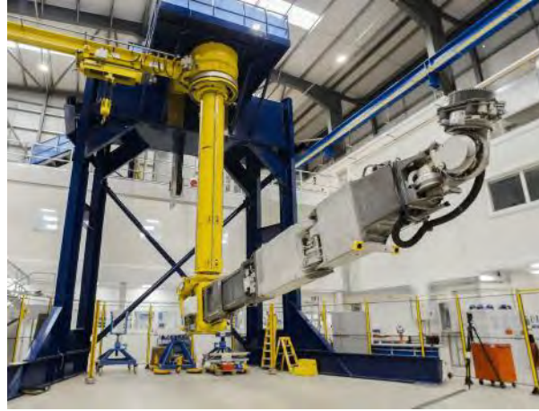
TARM remote operations integration test rig
