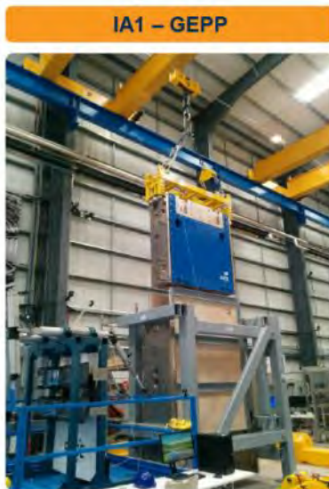
Compliance system for crane-guided insertion and removal
